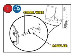
With someone supporting the Display and Accessory Hooks assembly, reconnect the Comm. Wire from the Display Mount to the Coupler.
