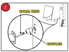
Disconnect the Comm. Wire that leads from the Display. Leave the Coupler connected to the Comm. Wire leading from the machine.
