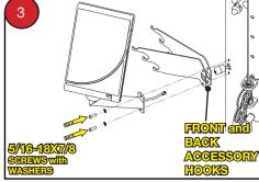
Route the Comm. Wire through the port hole of the Accessory Hooks. Align all screw holes and set two (2) 5/16"-18x7/8 Screw with Washer from the original screws through screw holes.
