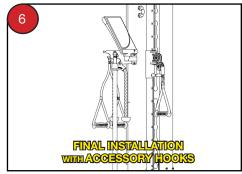
Check to ensure all Washers and Screws are fully seated and that there is no movement of the Display Mount and/or Accessory Hooks before operating the machine.
